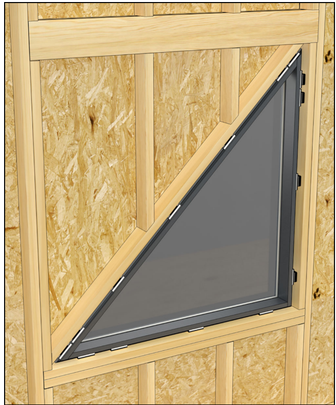
Figure 2 Example of bracing for polygon shapes.
