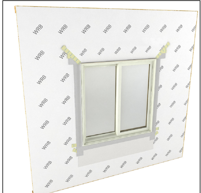
Figure 20 Sealing the Installation in air barrier applications.
