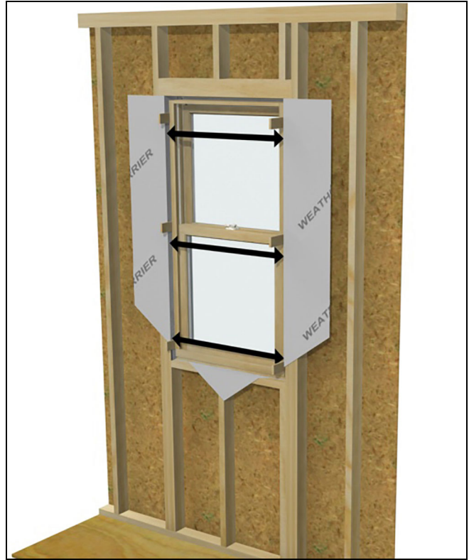
Figure 19 Measure at 3 points and adjust shims until equal.
