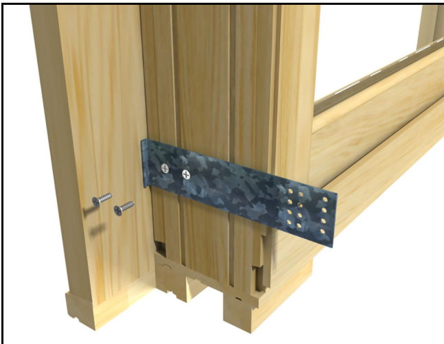
Figure 10 Apply brackets/clips to units with flat casing (if applicable).
