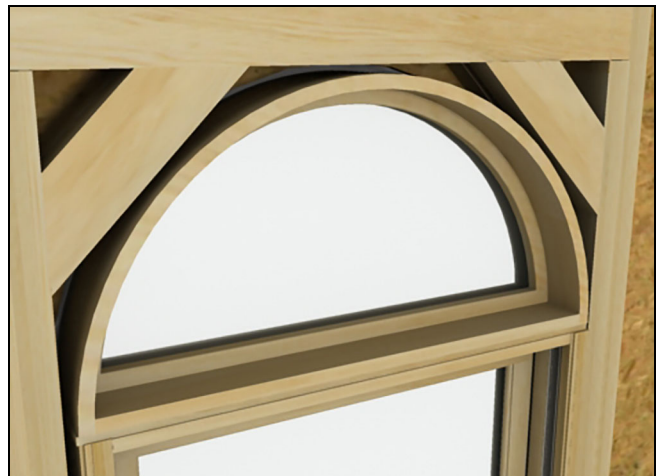
Figure 3 Typical rough opening for a round top.
