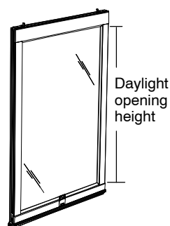
Top Sash Interior View
