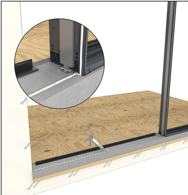
Figure 29 Sealing bead along sheathing line
