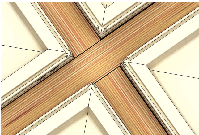
Figure 13 Notching detail for intersecting mulls
