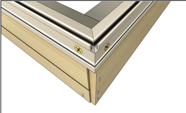
Figure 11 Close up of notched corner
