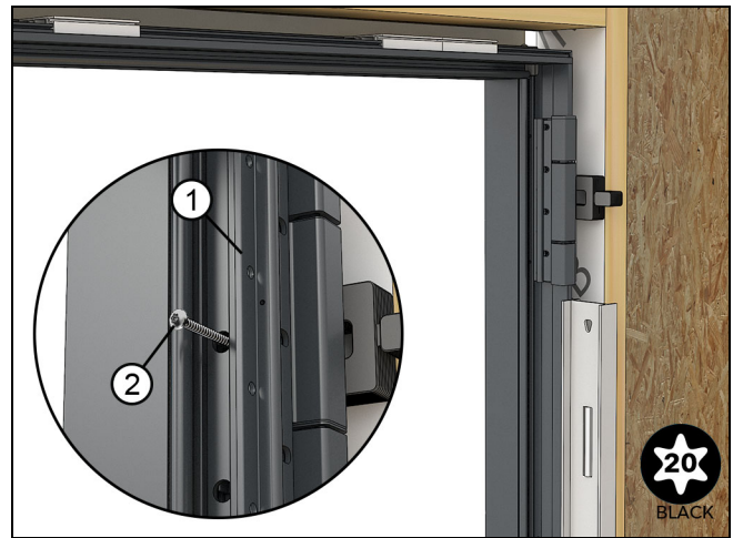
Figure 41 Plumb interior to exterior, shim and fasten
