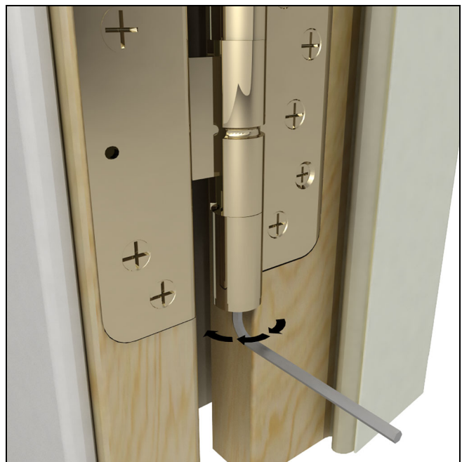
Figure 13 Lower the panel, counter-clockwise adjustment
