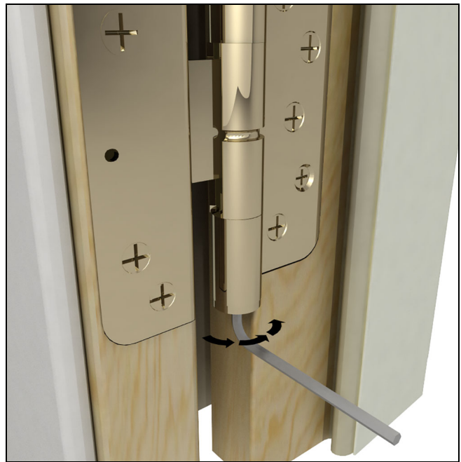
Figure 12 Raise the panel, clockwise adjustment
