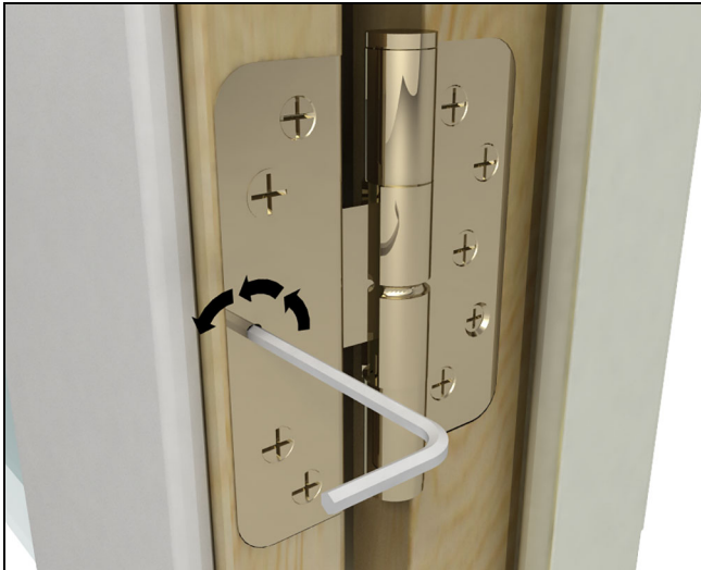
Figure 10 Counterclockwise to move panel away from jamb.
