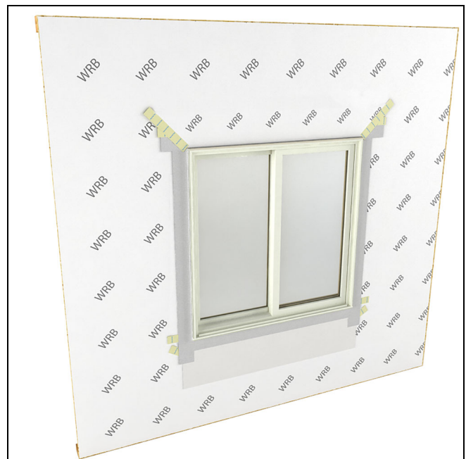
Figure 21 Sealing the Installation in air barrier applications.
