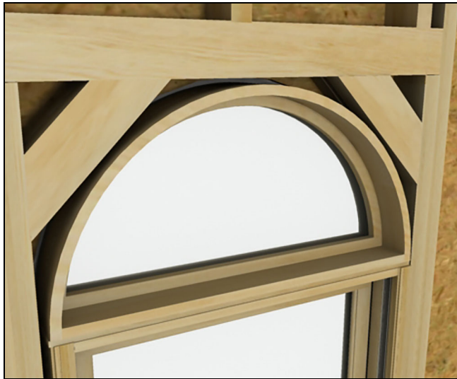
Figure 3 Typical rough opening.
