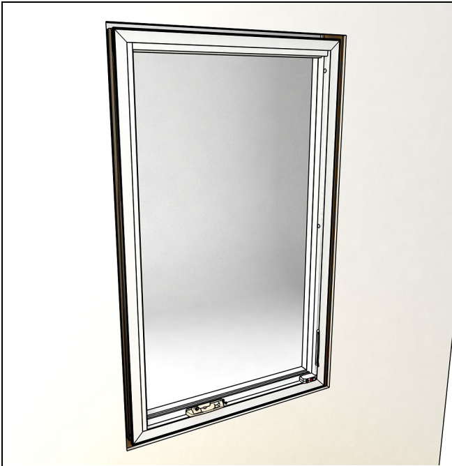
Figure 13 Completed casement unit with WOCD.
