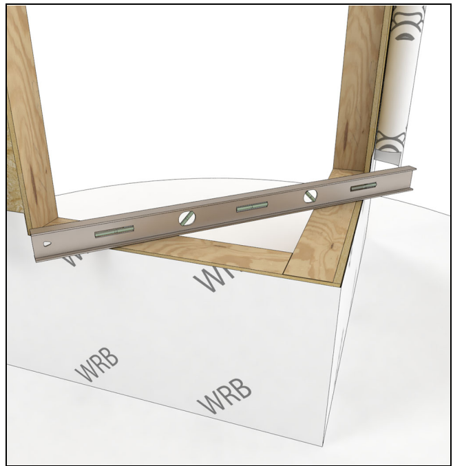
Figure 10 Check the sill for level
