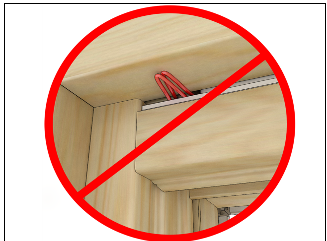
Figure 3 Make sure not to pinch wire leads between parts.
