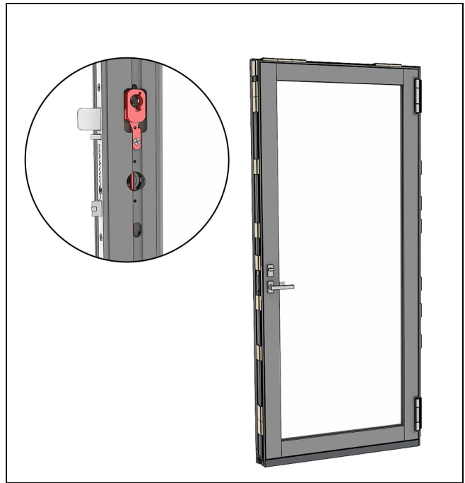
Figure 44 Swinging Door shown with cladding cut away
