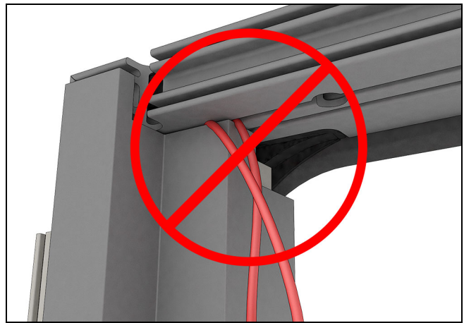
Figure 35 Make sure not to pinch wire leads between parts.
