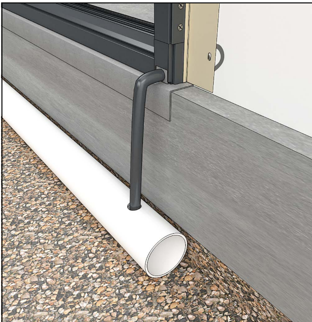
Figure 9 Weep tube terminating into drainage pipe
