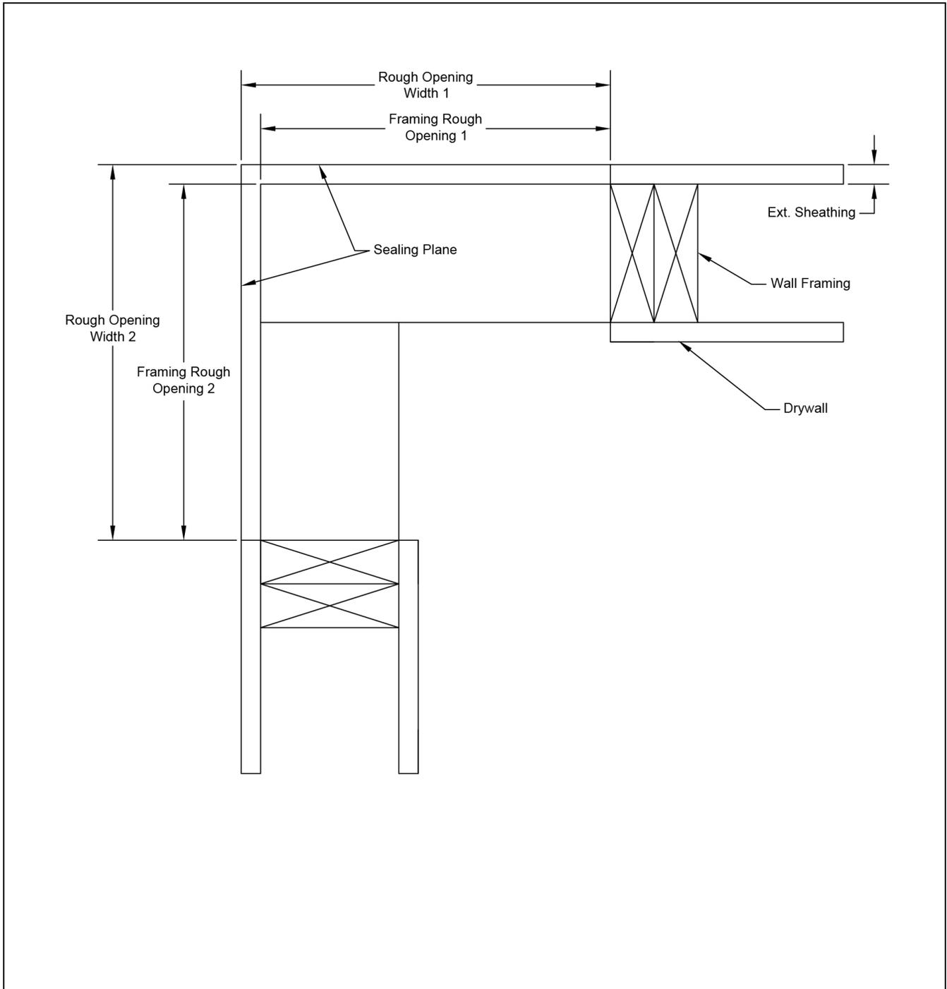
Figure 2 Framing Detail
