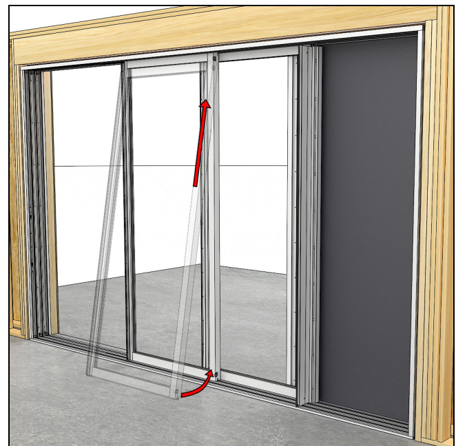
Figure 86 Install secondary operating panel
