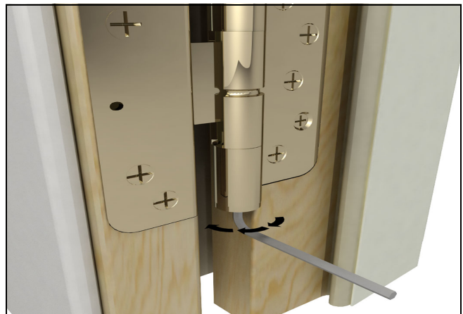
Figure 35 Lower the panel, counter-clockwise adjustment
