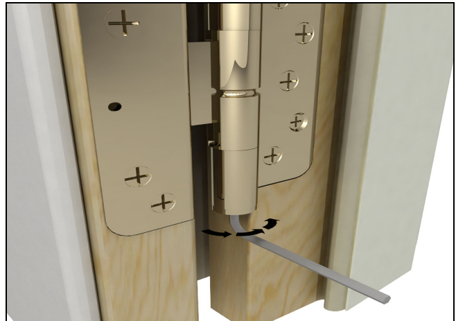
Figure 34 Raise the panel, clockwise adjustment
