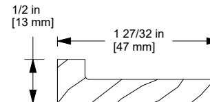
W2179, Sill Liner (Transom and Picture units) Ultimate Wood Double Hung Round Top Ultimate Wood Double Hung Magnum Round Top
